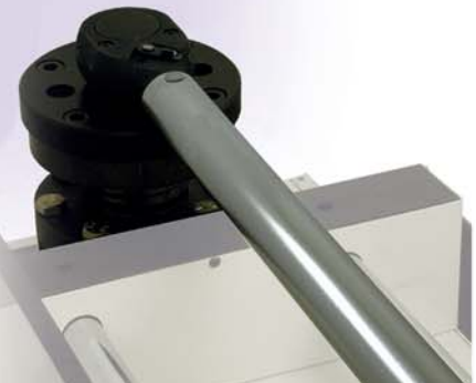
Tests and Calibrates Wrenches up to 2000 ft. lbs.
