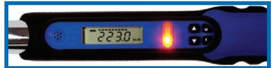
The yellow LED illuminates within 10% of target torque.
