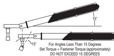
When using a universal or wobble extension, do not exceed more than 15 degrees & offset from perpendicular
