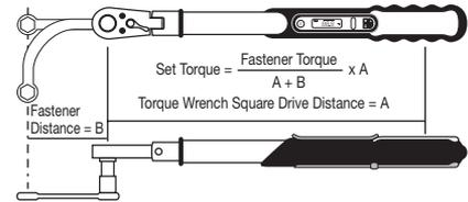
Fastener torque is greater than torque wrench square drive torque. Calculated setting will be lower than desired fastener torque.
