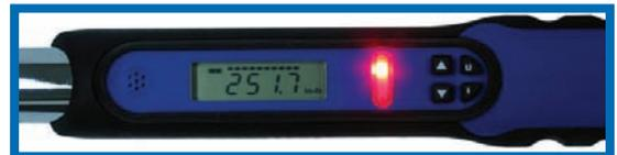
The red LED illuminates 4% beyond target torque, indicating fastener was overtorqued. Rapid “alarm” buzzer sounds.
