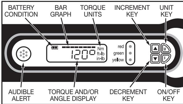
1. Turn the wrench **ON** by momentarily pushing the **ON/OFF** key. The display will return to the mode of operation and preset values previously set up.
