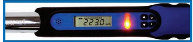
The yellow LED illuminates when the applied torque value equals -10% of the target torque value.
