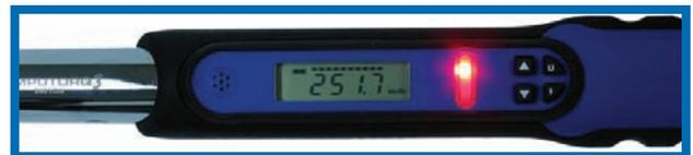
The red LED illuminates at +10% of target torque, indicating fastener was overtorqued. Rapid “alarm” buzzer sounds.
