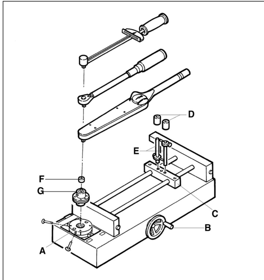
Figure 6-2: 2000-600-02 Manual Loader, Exploded View
