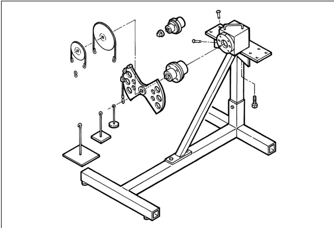
Figure 5-2: Single Low Torque Transducer Mounting Detail
