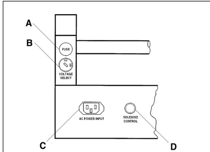
Figure 6-3: 2000-600-02 Manual Loader Rear Panel Controls
