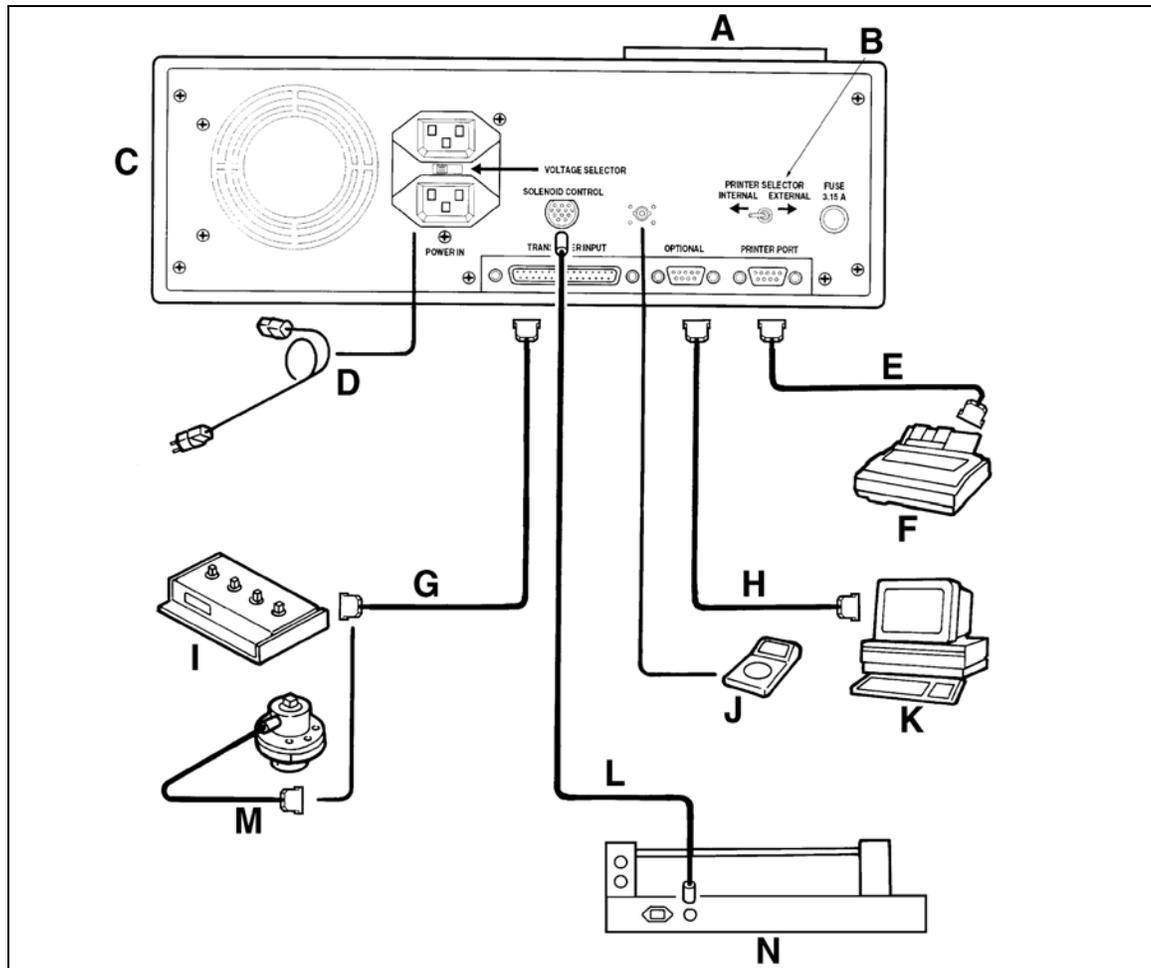
Figure 3-1: MULTITEST Torque Tester/Calibrator/Loader Setup
