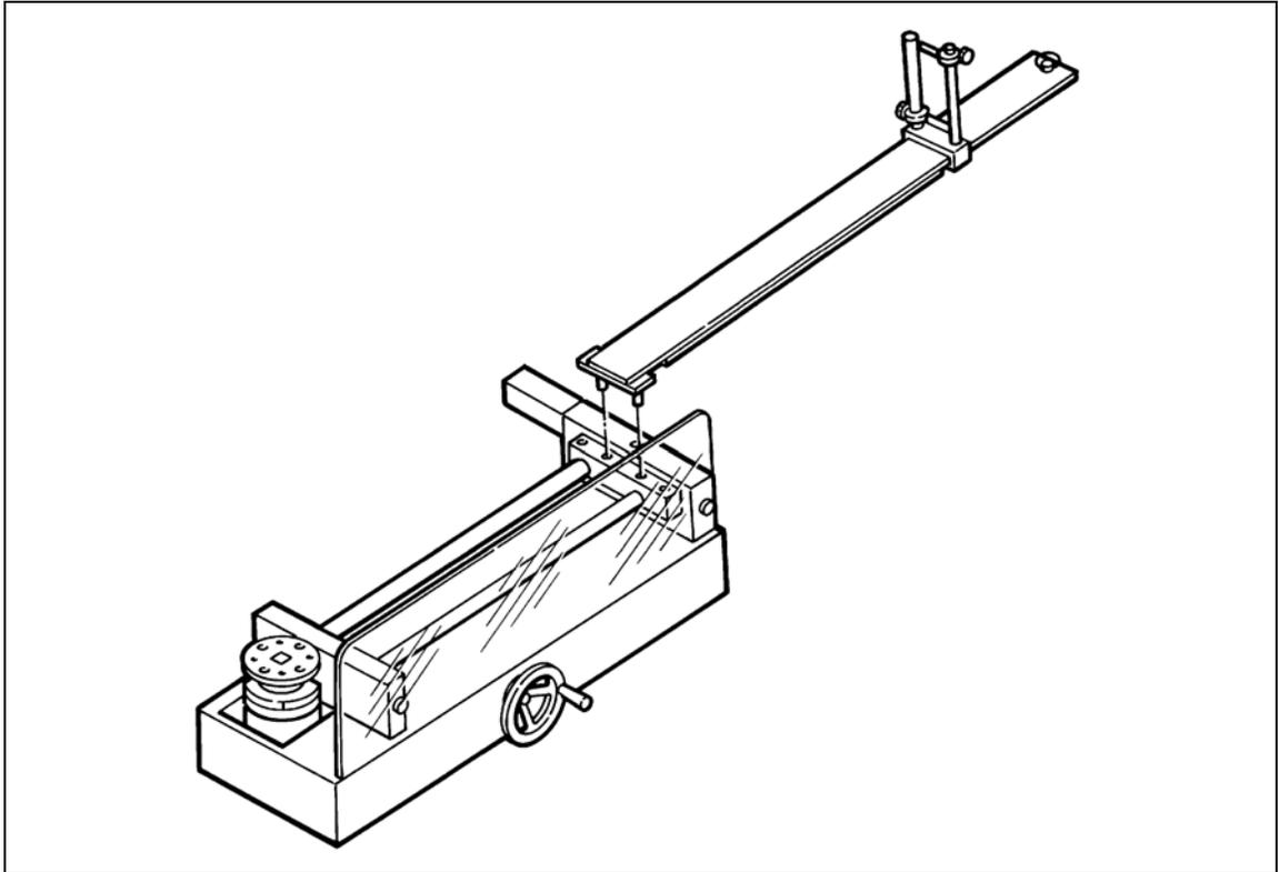
Figure 6-6: 2000-600-02 Manual Loader Extension Arm
