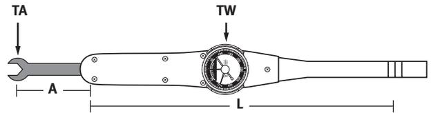
A number of variables can affect torque accuracy. These include the length of an adapter or extension, length of the wrench and variations in hand position on the wrench will affect the accuracy of the above calculation.
