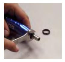
3. Replace the cone nut and tighten counterclockwise. Then tighten the cone nut to  $80\pm3$  IN.LB.
