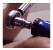
7. Use a 1/16" hex in a screwdriver to loosen and remove the 2 (two) screws on the scale bezel. Remove the bezel. Move the scale until the increment line is aligned to the lowest increment.
