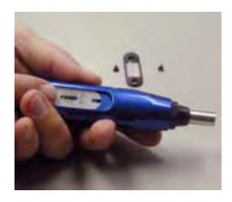
8. Place the Bezel over the scale and tighten the screws. Recheck the readings at 20, 60 and 100% of scale. If the screwdriver is calibrated torque the Bezel screws at 3±.2 IN.LB. Then the set screw to 60±2 IN.LB. Place a new end plug on the end of the screwdriver.
