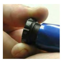
6. Place the 1/8" T-Shaped Hex in the back of the knob and Loosen the set screw. Pull the knob back and turn it until it is on the "0" increment of the knob is aligned with the 20% increment of the scale. Push the knob back to engage it and tighten the set screw. Recheck the reading.
