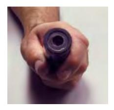
5. Test the screwdriver and Adjust the handle, clockwise to increase and counterclockwise to decrease the reading, until the screwdriver read within specification of the 20% reading (example: For a 100 IN.OZ. CDI screwdriver, the low reading is 20 IN.OZ. and 18.8 to 21.2 IN.OZ. is the tolerance).
