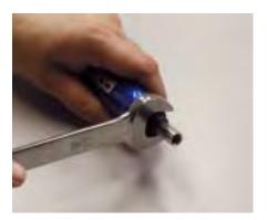
2. Turn the cone counterclockwise to the remove from cone from the screwdriver.
