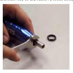
3. Remove the cam from the screwdriver.
