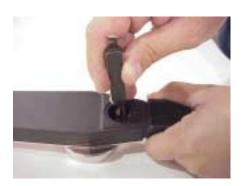
The Dial Wrench Adjusting Tool (Part # 600-2) allows adjustments to be made in small, slight movements. The adjustments to the push rod must be made in very small increments, generally not to exceed .010 (.26mm). Test the wrench on a torque tester after each incremental adjustment.
