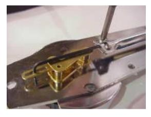
Then loosen the screws on the channel. Every 0.010 increase or decrease of the distance will change the reading value approximately 3 to 6 %. After moving the push rod, tighten the channel screws, re-assemble with the case and test the readings.
