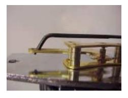
If the push rod is bent up so far as to be coming out of the loop of the movement.
