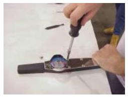
After removing the case measure the distance between the push rod bent end and the end of the movement loop, with the inside diameter end (blades) of a caliper.
