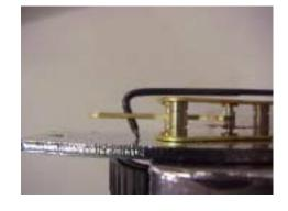
Use the Dial Wrench Adjusting Tool (Part #600-2) and gently move the push rod until it is centered to the channel and in the movement loop and not touching the plate Next, perform an accuracy check.
