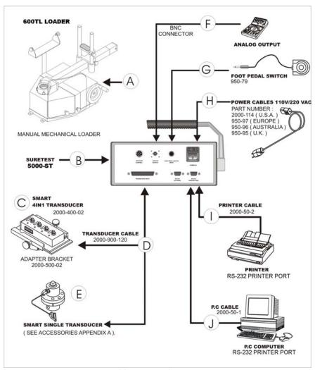
Figure 3-1: CDI 5000-3 Torque Tester/Calibrator/Loader Setup
