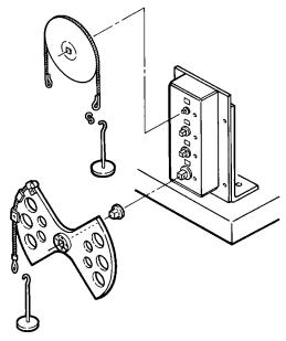
Figure 5-3: 4-in-1 Transducer Mounting Detail
