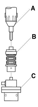
Figure 4-1: Power Tool Test Setup
