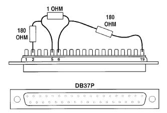
Figure 5-2. Calibration fixture
