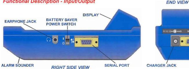
BATTERY SAVER POWER SWITCH - Disconnects the rechargeable battery from the MULTITORQ<sup>™</sup> circuit. At power-on. unit comes to life, self-checks and returns to last SET-UP parameters unless sensor has been changed.
